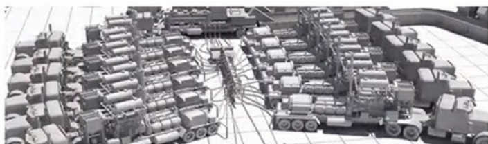
Status Quo Pumping Model with 15-20 PD Pumps
