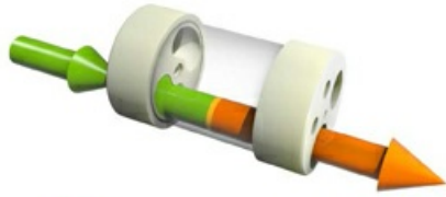
1 Low-pressure feed water fills rotor chamber, displacing brine
