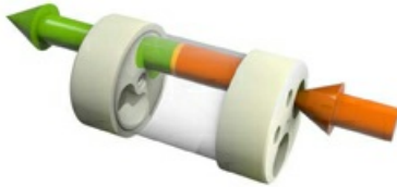
3 High Pressure brine pressurizes and displaces feedwater
