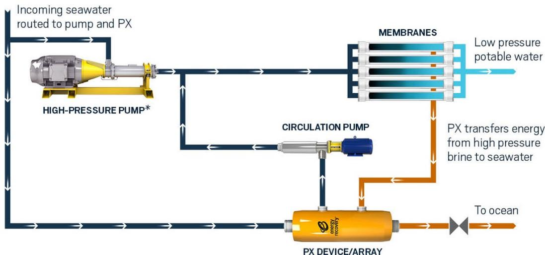
\* Main pump size reduced by up to 60% compared to a SWRO process not using any energy recovery device.
