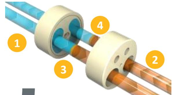
3. Low pressure driven fluid contacts motive fluid, expelling it at low pressure
