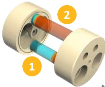
1. Low pressure driven fluid that will be pressurized and sent into system
