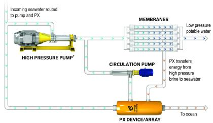
Main pump size reduced by up to 60% compared to a SWRO process not using any energy recovery device. Table of Contents
